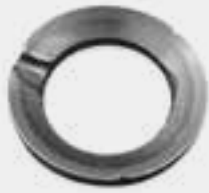
eroded ball seat
